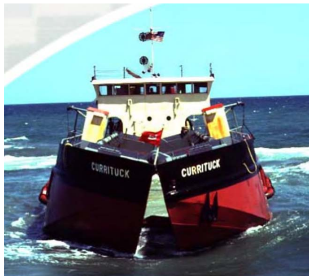
Figure 2-9. USACE Shallow Draft Split-Hull Hopper Dredge the Currituck Rarely Dredges the LWF Inlet
