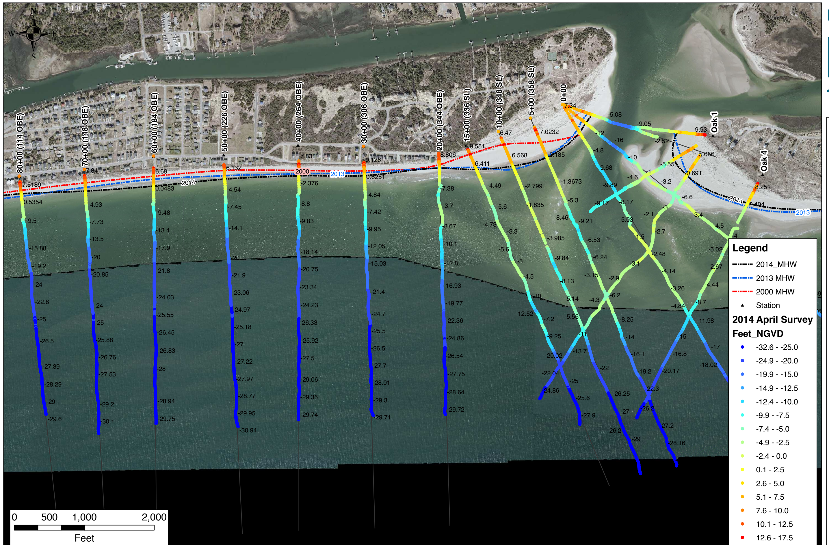
FIGURE B-1 April 2014 Survey Data: 2014 Mean High Water (MHW) Shoreline, 2013 MHW Shoreline and 2000 MHW Shoreline on 2012 Aerial.
